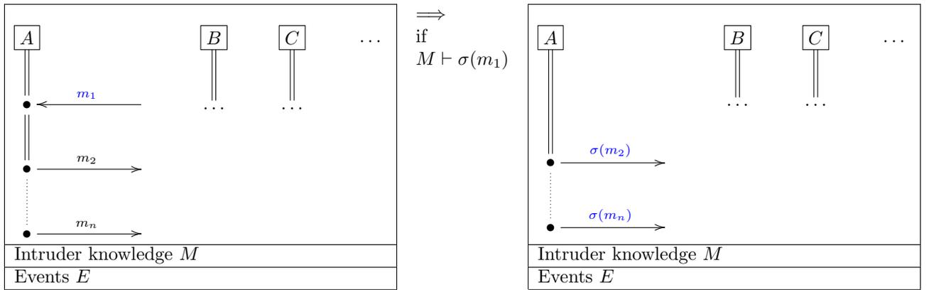
The substitution  $\sigma$  is applied to the rest of the strand since all variables that have been bound by the receive step are bound to that value for the rest of the strand. Again this reflects the fact that the intruder controls the network: all messages that an honest agent receives come from the intruder. Observe that the strands do not carry any information about who the claimed sender is, since the intruder could anyway insert any name he knows.
