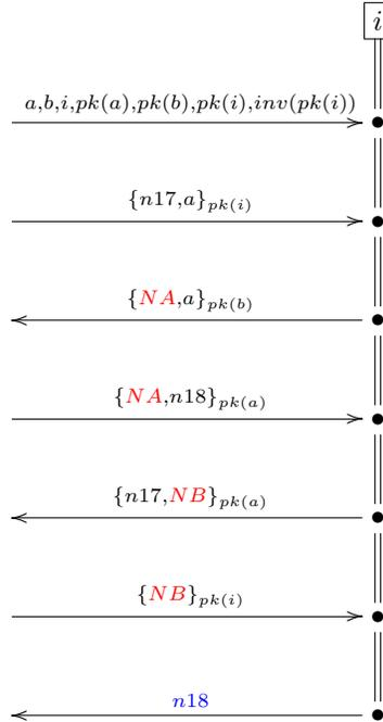
In section 13 we give a decision procedure for such constraints. In fact there is a solution for this example (and only one):  $\sigma(NA) = n17$  and  $\sigma(NB) = n18$ ; that's the secrecy attack from Example 13.  $\square$
