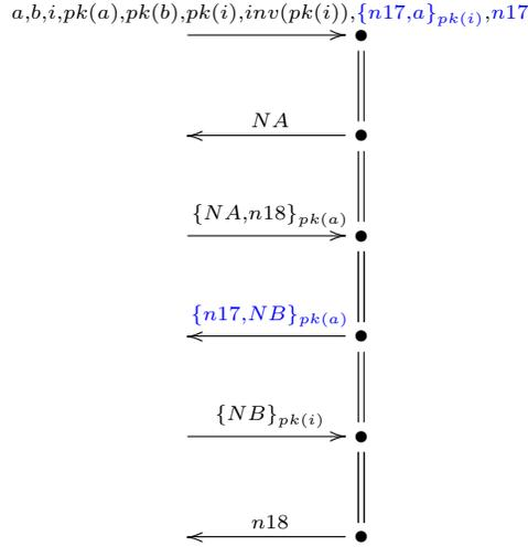
We can apply unification between the incoming message  $\{n17, NB\}_{pk(a)}$  and the outgoing message  $\{NA, n18\}_{pk(a)}$ . The unifier (according to the mgu algorithm) is  $\sigma = [NA \mapsto n17, NB \mapsto n18]$ . We apply it to entire constraint and remove the outgoing message we have just “done” by unification:
