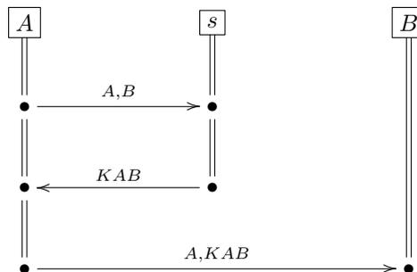
Similarly, an attack trace can be represented by a message sequence chart, for instance using the OFMC option `--attacktrace`, an SVG file is created containing the attack as an MSC.
