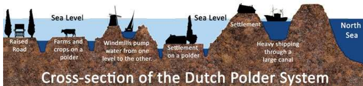
Fig. 16.7 The Dutch Polder System
