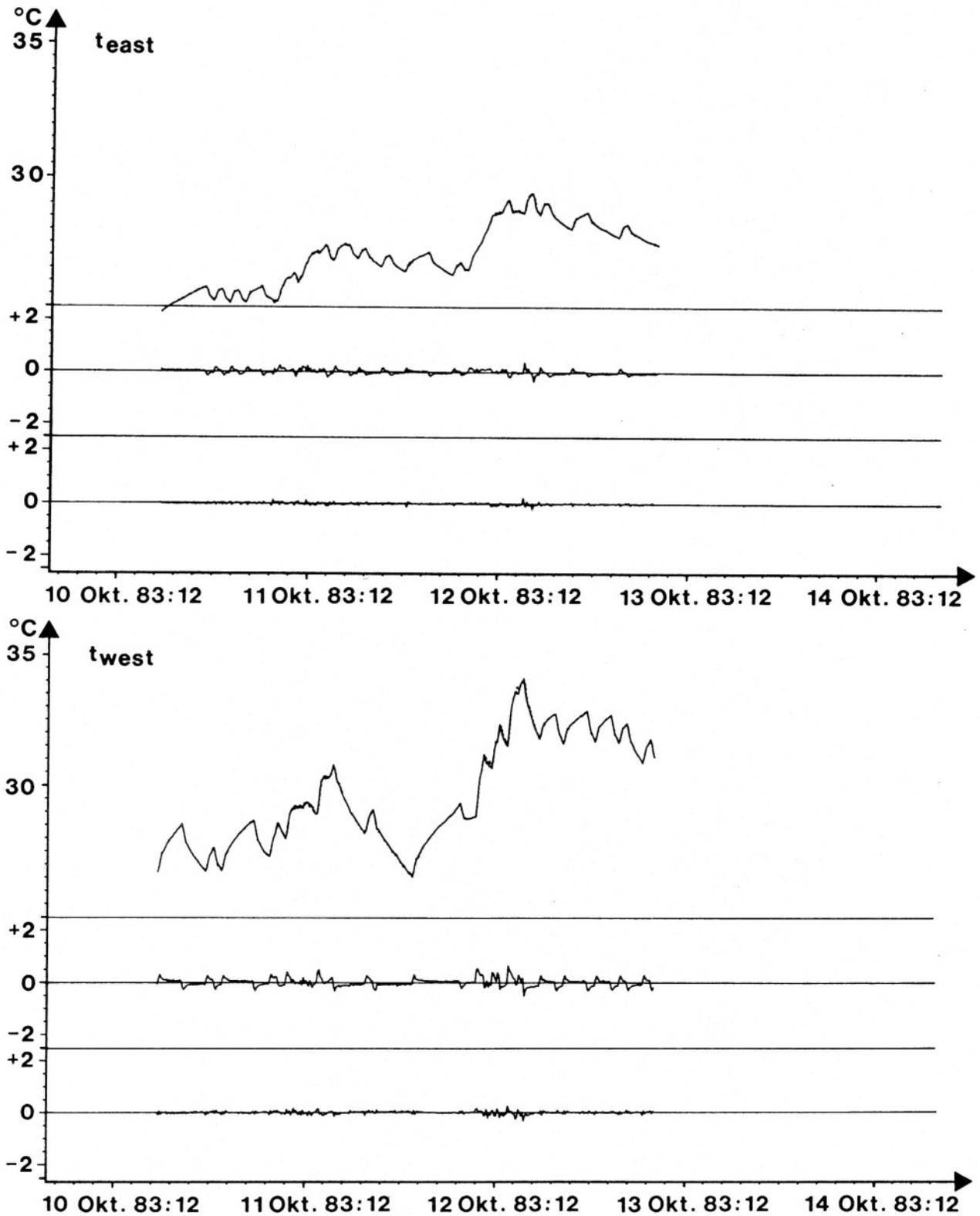
Figure 3. Measured and estimated indoor temperatures, the measured ones differenced once and the residuals from the 'full model'.
