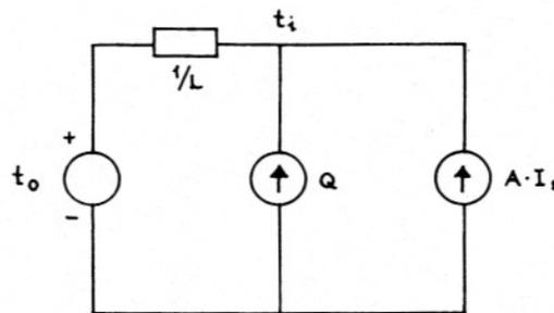
This model does not take the heat capacity of the house into account. For dynamic analysis, the following model is better, see also Sonderegger, 1978 /3/ or Oldengarm and Euser, 1981 /4/:
