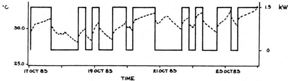
Figure 1. Example of a PRBS with  $n=4$  and  $T=5$  hours.
