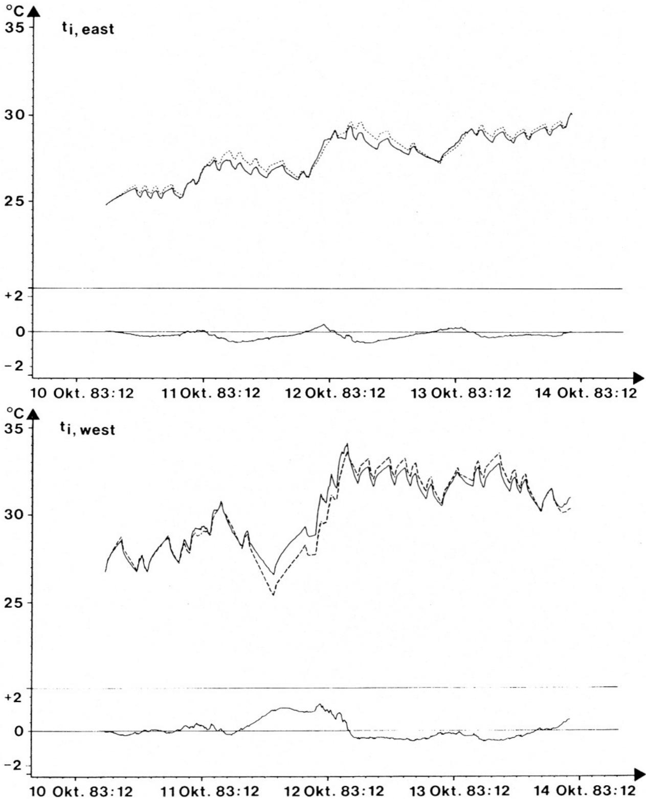
Figure 4. Measured and simulated indoor temperatures, and the differences between the two.
