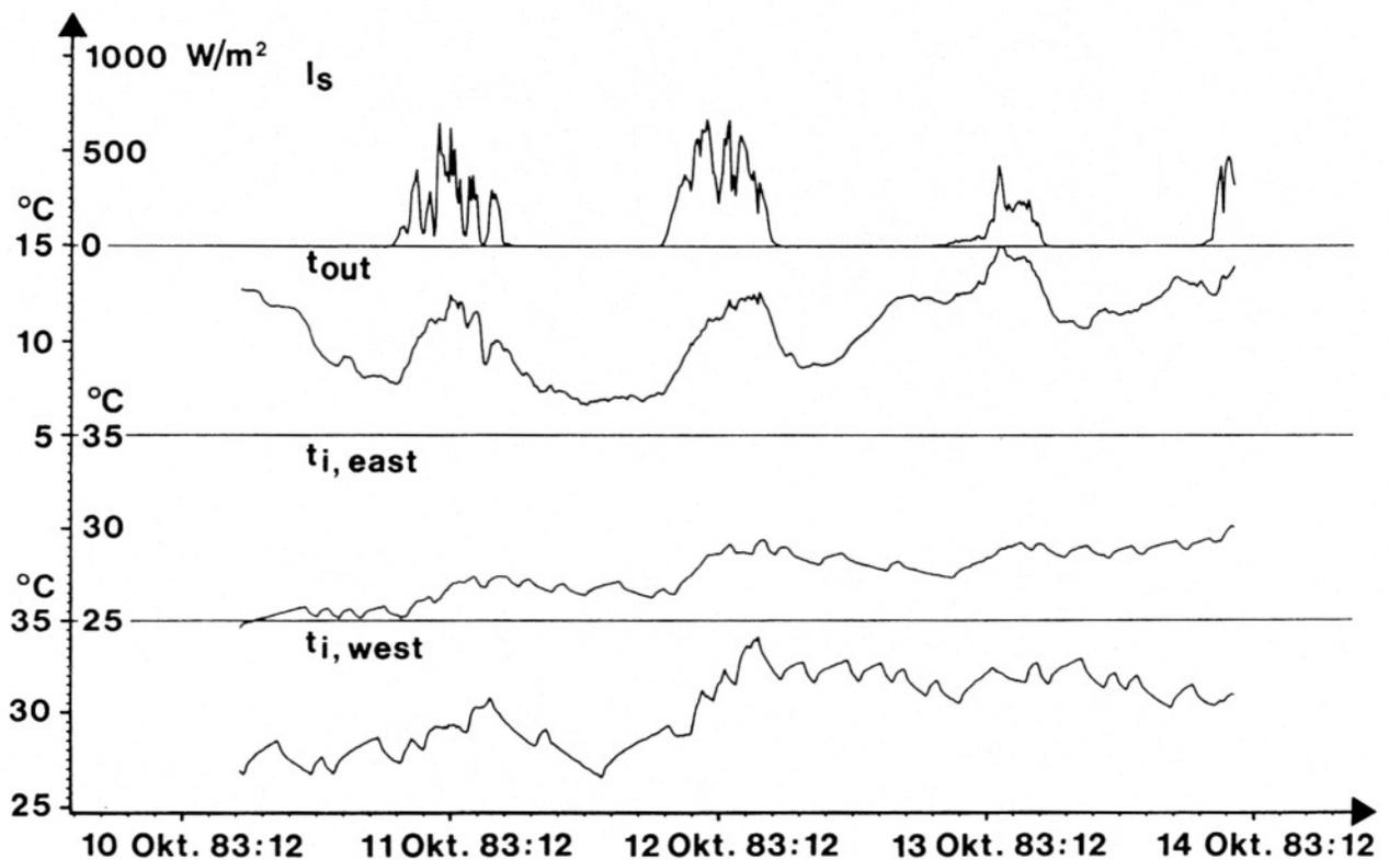
Figure 2. Data from both rooms of the low-energy test house and outdoor parameters. Scans every 10 minutes. PRBS not shown.
