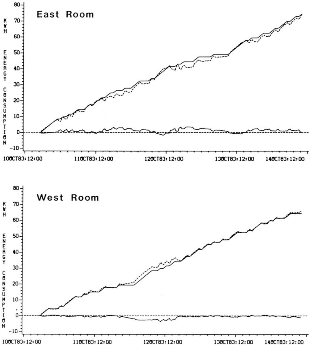
Figure 3. Measured and simulated cumulative energy consumptions and the differences between the two using the model described by Equation 3 with the parameters from Table 1 (omitting  $H$  in the simulation process).
