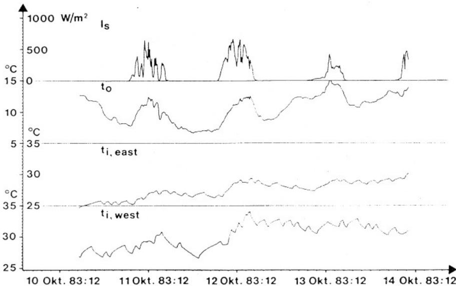
Figure 2. Data from both rooms of the low-energy test house and outdoor parameters. Scans every 10 minutes. PRBS not shown.
