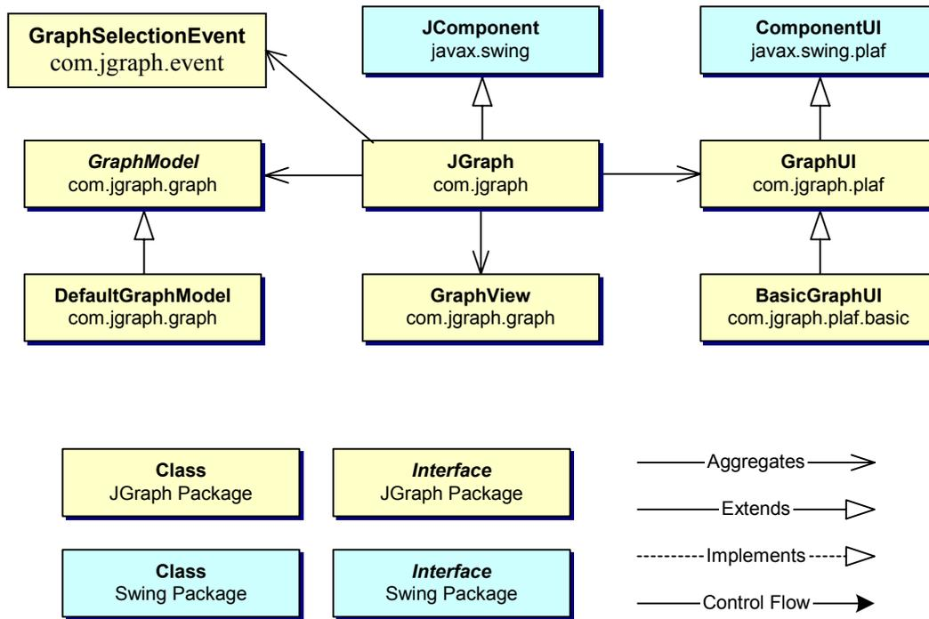
Figure 18. JGraph MVC in UML
