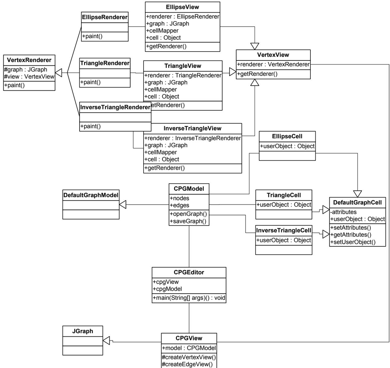
Figure 22. UML class diagram for CPG editor
