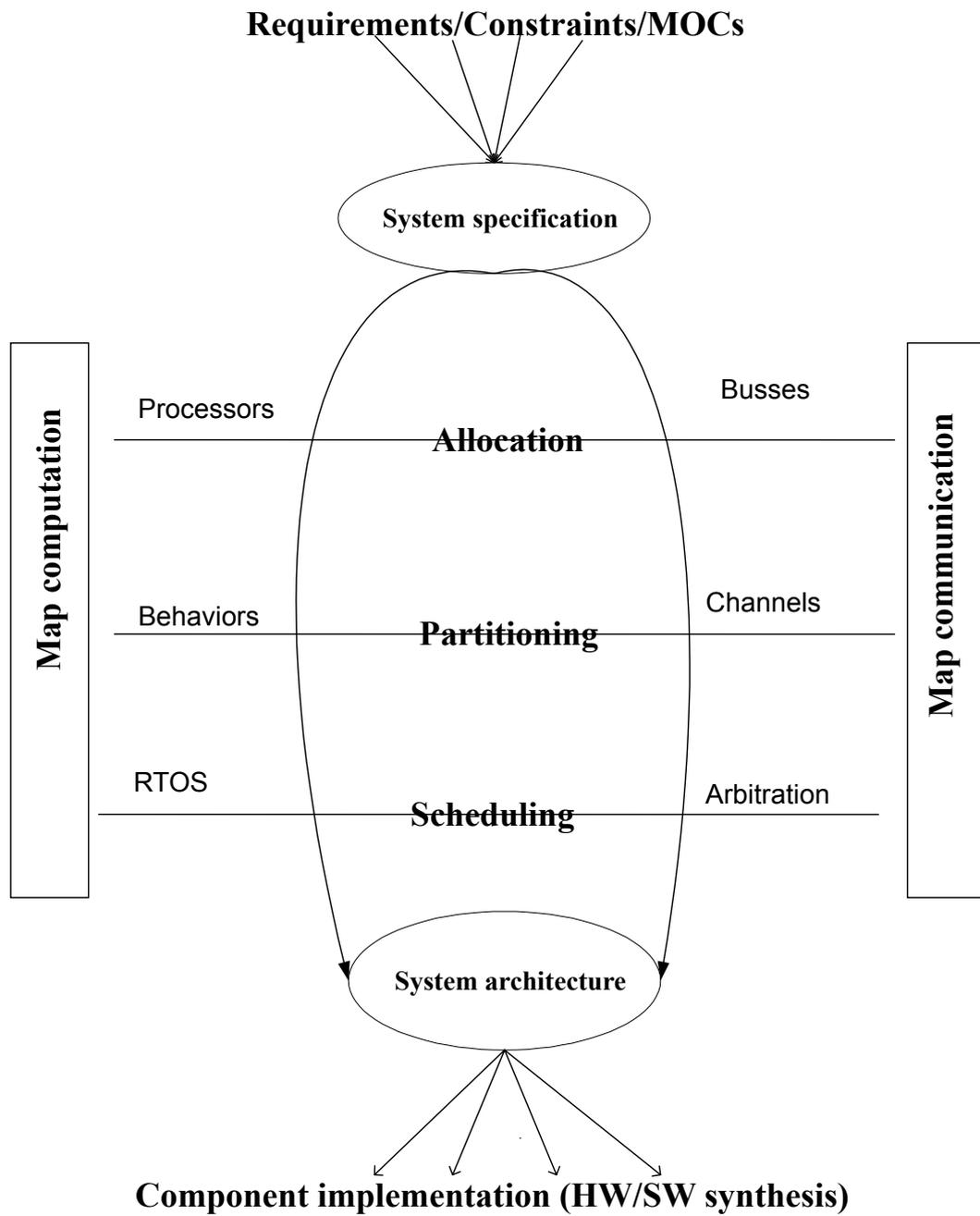
Figure 1. Embedded system design tasks
