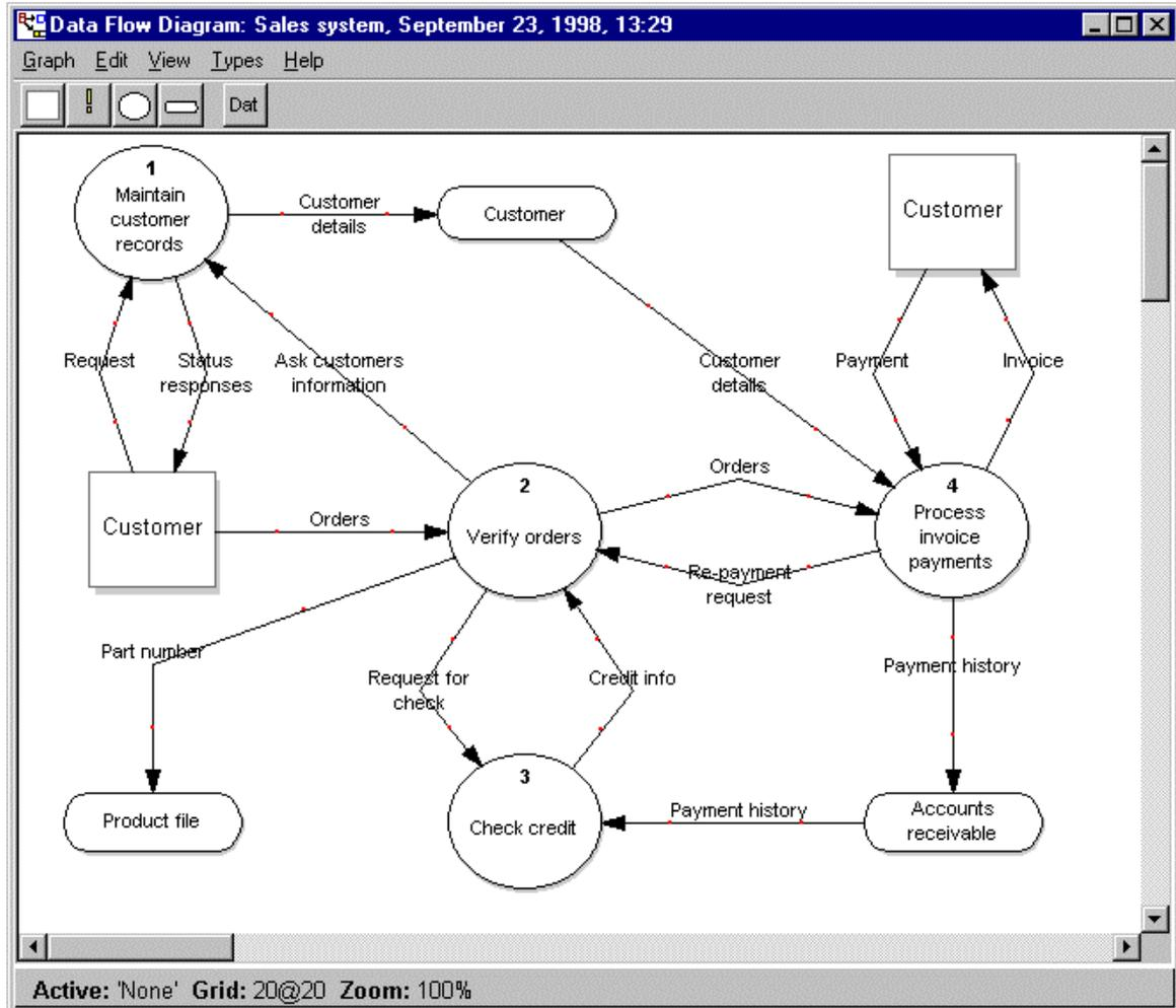
Figure 11. Data flow diagram editor
