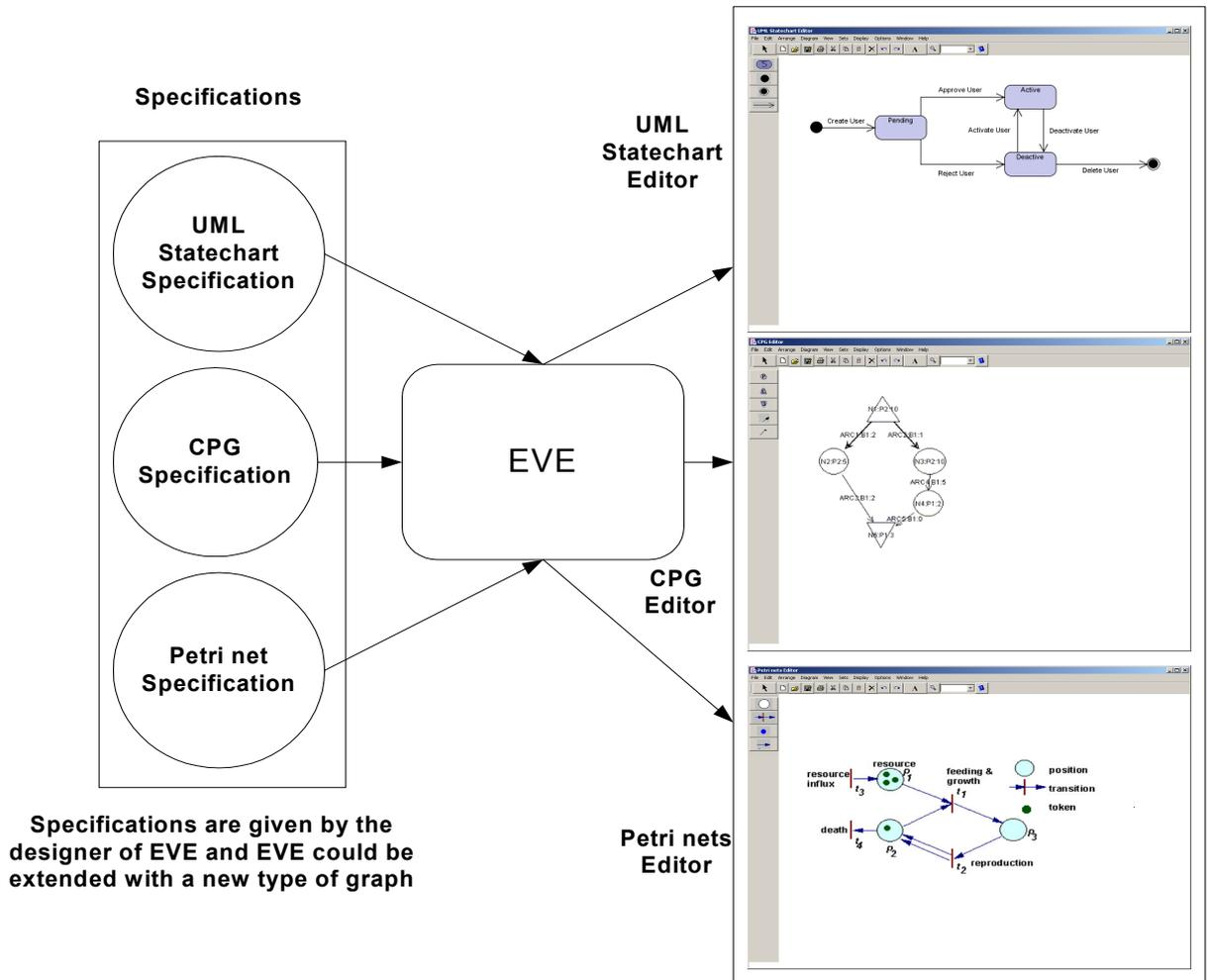
The three models are from respective graph files that written based on the specifications and describe parts of an embedded system
