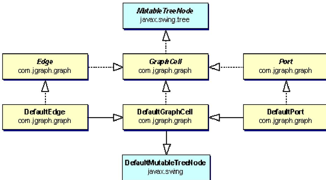
Figure 19. GraphCell interface hierarchy and default implementations
