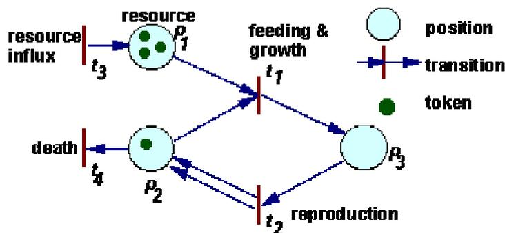
Figure 6. Example of a petri net
