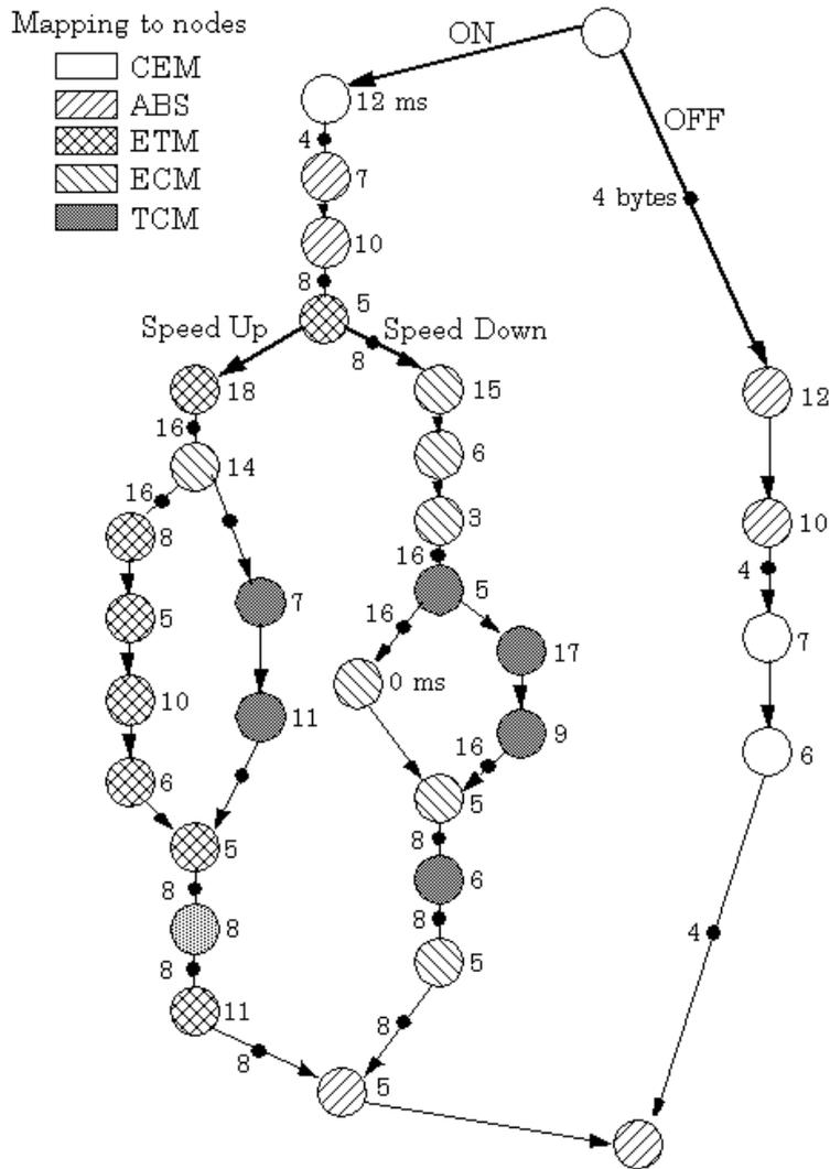
Figure 5. The cruise controller behavior
