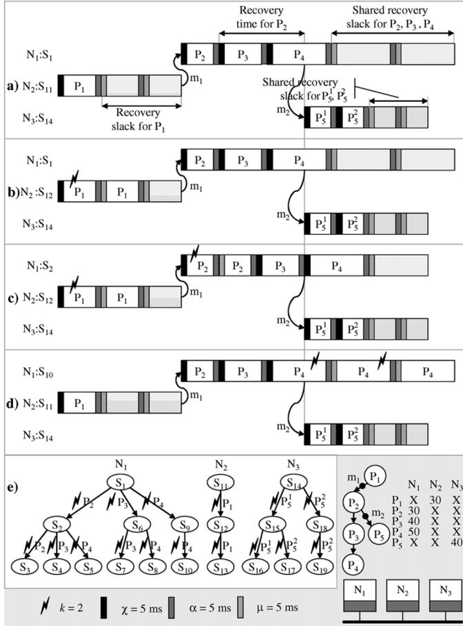
Fig. 3. Fault tolerant scheduling example. The initial schedules (corresponding to the no-faults scenario)  $S_1$ ,  $S_{11}$ , and  $S_{14}$ , for each node, are the root schedules. If a fault occurs in  $P_1$ , we switch from  $S_{11}$  to  $S_{12}$  on  $N_2$ , but  $S_1$  and  $S_{14}$  on  $N_1$  and  $N_3$ , respectively, are undisturbed because the fault occurring on  $N_2$  is transparent to  $N_1$  and  $N_3$ .
