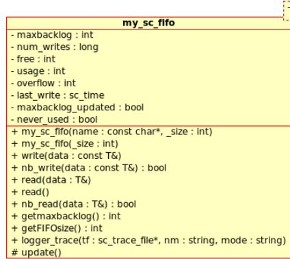
**Figure 5.2:** Class diagram of the modified `my_sc_fifo` class, which is used instead of the standard SystemC FIFO buffer.
