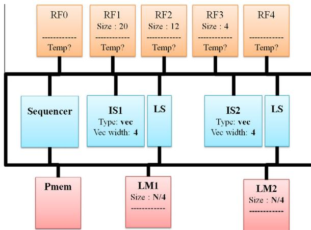
**Fig. 8.** Example of selected ASIP architecture. The number of allocated registers is equal to the number of the allocated issue slots. However, some register sizes are not known because their final value is computed from the subsequent phase 3.
