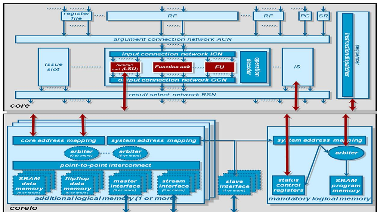
Fig. 1. Generic ASIP architecture of the targeted MPSoC platform.
