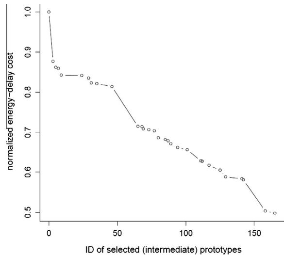
Fig. 13. Set of 31 candidate architectures for rapid prototyping, automatically selected by phase 3 after considering 186 alternative architectures in its design space.
