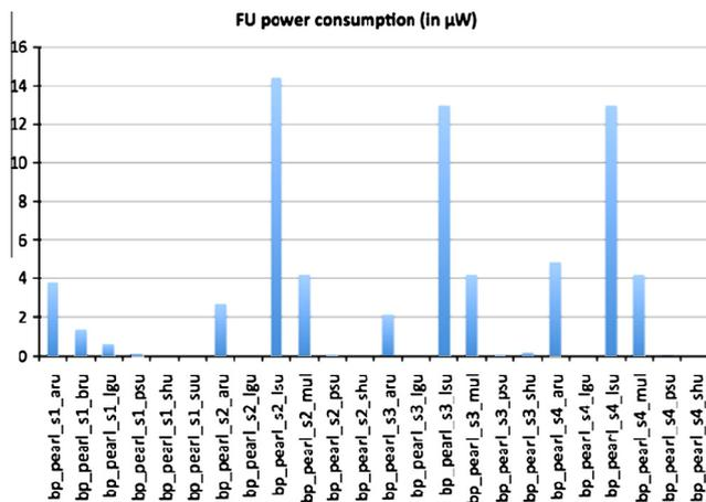
Fig. 15. Power consumption for each FU in a particular configuration, composed of four issue slots, with register files of 16 entries, reported in  $\mu\text{W}$ . As can be seen from graph, load-store units and arithmetical units are the power hot-spots in the design.
