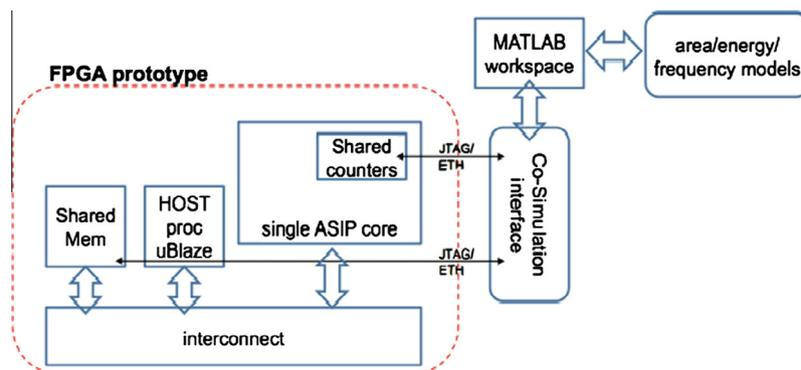
Fig. 9. Block diagram for FPGA/MATLAB SysGen interfacing.
