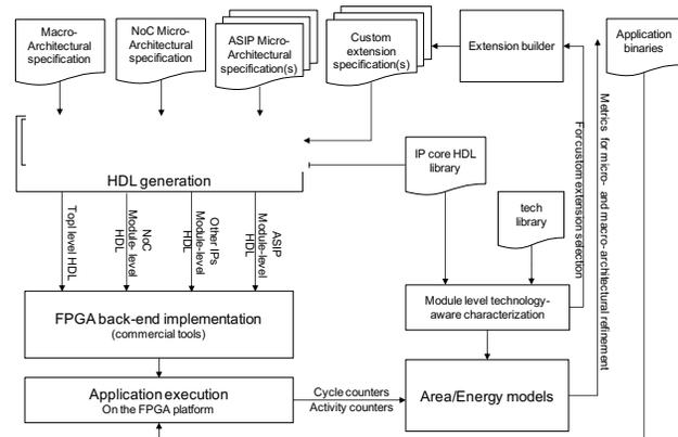
Figure 5 FPGA prototyping
