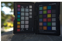
Figure 4. Photos of Xrite ColorChecker are used to calibrate color between main camera Sony A7 and envmap camera Insta360 Pro2
