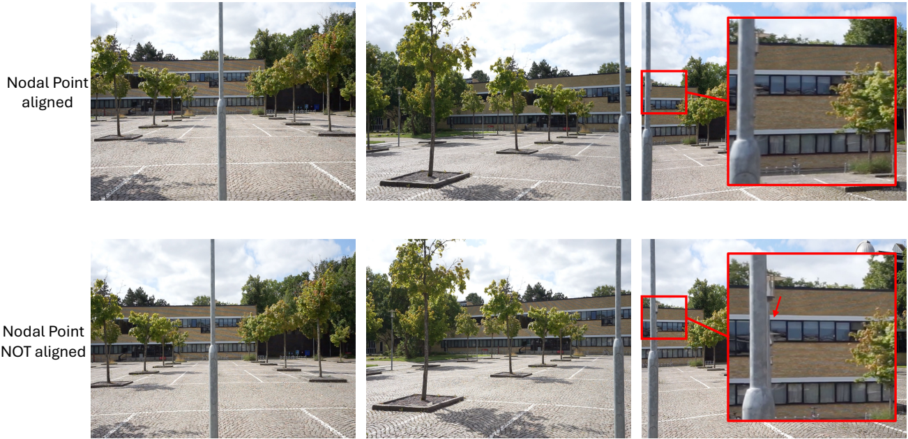
Figure 12. Nodal point alignment. When the camera is not positioned at the nodal point, rotating the camera causes the nearby utility pole to fail to occlude the poles behind it. In contrast, when the camera is at the nodal point, the nearby utility pole can occlude the poles behind it.
