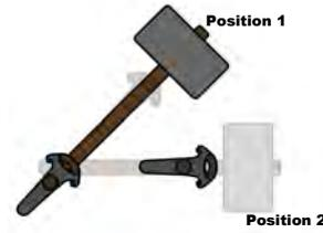
Figure 7: Hammer chasing the controller during rotation. Rotation is delayed when user motion is too quick, so that the hammer needs a brief moment of slower user motion to catch up with the controller closest to the hammer head.
