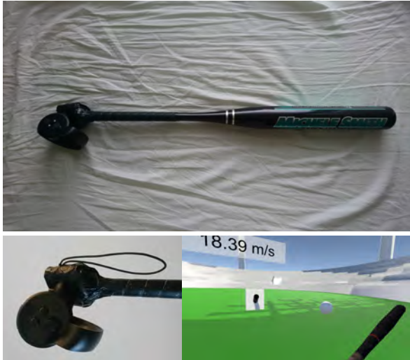
Figure 16: An Oculus Touch controller attached to the base of an aluminum baseball bat. We use this aggregate in a test conducted in a crude stadium scene with a pitching machine.
