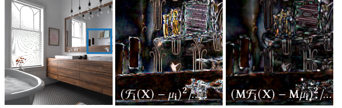
Figure 4: Comparing relative squared error with (right) and without (middle) incorporating spatial contrast sensitivity, as described in Sec. 3.2. The modified metric places less emphasis on error that is not perceptually relevant under regular viewing conditions, such as along edges and fine details that are not easily perceived in the denoised image (left).
