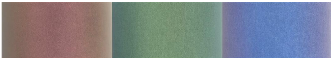
Figure 1 Photographs of inks prepared with nominal Red (left), Green (middle) and Blue (right) pigments. Inks were applied on black paper and wrapped around a cylinder under diffuse daylight illumination.
