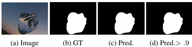
Figure 5: Prediction of segmentation masks: (a) input image, (b) ground truth mask used for comparison, (c) predicted mask with decimal values, (d) binary mask using values with certainty above 0.9.
