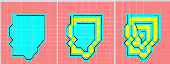
Toolpath generation with contour detection. (Fig.2)
