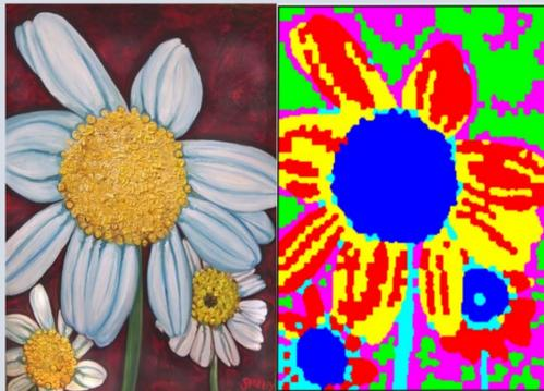
Color threshold based segmentation with superpixels in order to remove spare pixels (Fig.1)
