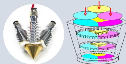
Nozzle tip diamond hot-end and cross section (Fig.5)
