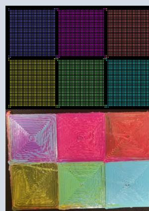
G-code points of six squares in the visualization tool (top). Six 3D printed squares without purge tower (bottom) (Fig.6)
