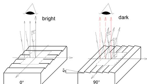
Figure 2. Demonstration of orthogonal contrast generation.
