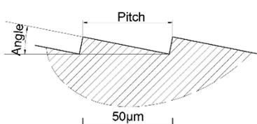
Figure 1. Anisotropic structure geometry: definition of pitch and angle.
