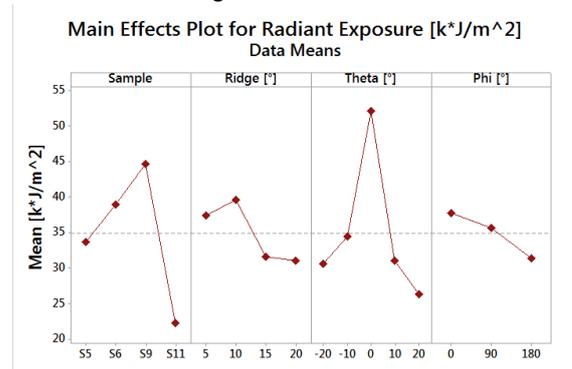
**Figure 3.** Main effects plot for the absolute reflectance. The name of the samples are listed in Table 1. Theta refers to the tilting angle of the microscope. Phi refers to the rotation angle of the sample.
