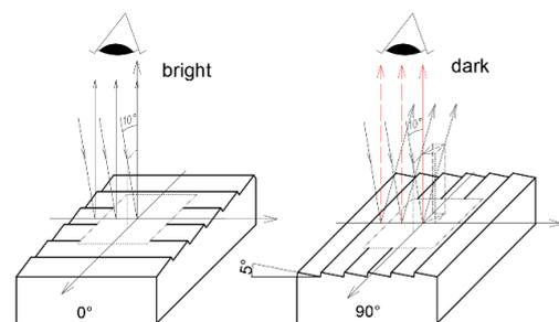
Figure 2. Demonstration of orthogonal contrast generation.
