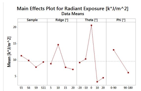
**Figure 4.** Main effects plot for the contrast. The name of the samples are listed in Table 1. Theta refers to the tilting angle of the microscope. Phi refers to the rotation angle of the sample.
