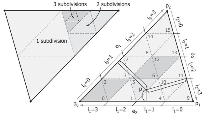
Fig. 6 Our indexing scheme for a volumetric layer.
