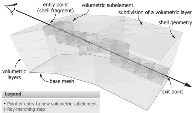
Fig. 4 The ray marching in step 5 of our shader pipeline.
