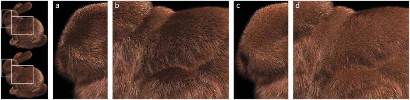
**Fig. 11** Comparison of explicit fur and hybrid fur. Magnified nose and back of the furry Stanford bunny seen in full in the leftmost column: **a, b** explicitly rendered fur; **c, d** hybrid rendered fur.
