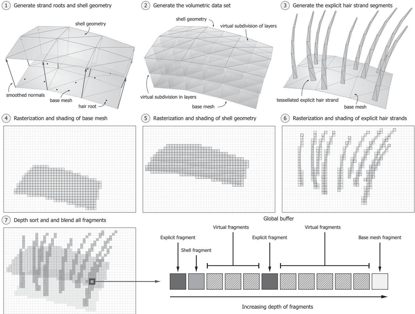
**Fig. 3** Overview of our shader pipeline. In steps 1–3, we generate explicit hair strand and shell geometry. In steps 4–6, the generated geometry is rasterized and shaded (see also Fig. 4 and Section 3.1-3.2). In step 7, the shaded fragments are depth sorted and blended in accordance with our blending algorithm (see also Fig. 5 and Section 3.3).
