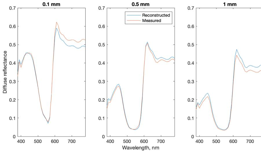
Figure 4: Comparison of the reconstructed diffuse reflectivity and the originally measured one for samples of the thickness of 0.1, 0.5 and 1 mm on white diffuse background.
