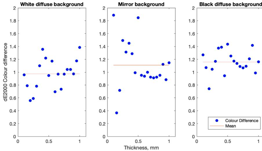
Figure 5: Colour difference between measured and reconstructed reflectivity values for all three backgrounds and each sample.
