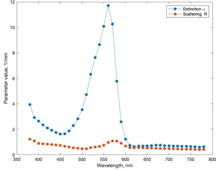
Figure 3: Effective extinction  $\alpha$  and reduced scattering coefficient  $R$  obtained from the fit.
