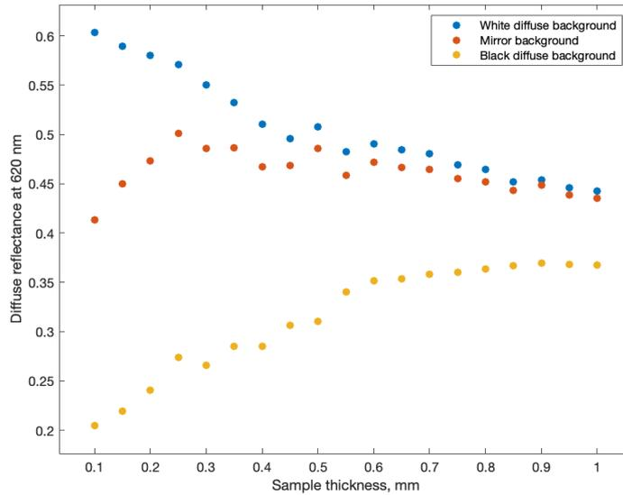
Figure 2: Diffuse reflectance at 620 nm with increasing sample thickness for all three backgrounds. As the thickness of the sample increases, the contribution of the background becomes less evident, and the values slowly approach a common saturation point.
