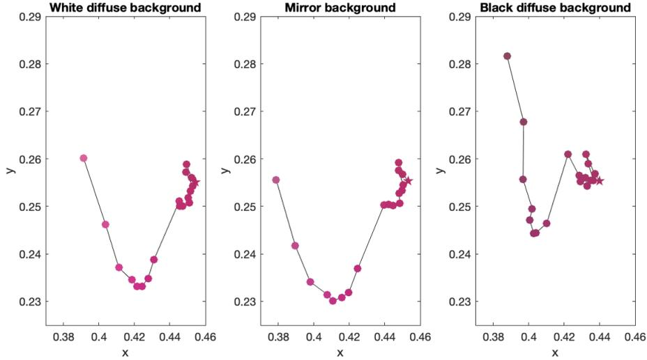
Figure 2: CIE  $xy$  chromaticity diagrams representing measured colour of the samples of Neon Pink filament of thickness 0.1 mm to 1 mm in steps of 0.05 mm. Coordinates correspond to the CIE  $x$  and  $y$  values. The colour of the points represents RGB values calculated from the measured diffuse reflectance values. Data for the 1mm thick sample are marked with a star.
