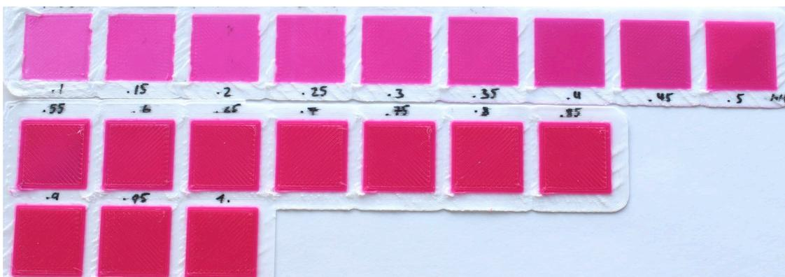
*Figure 1: Printed samples of Neon Pink PLA of thicknesses 0.1 to 1 mm photographed on a white background. Because of the material translucency, the background is affecting the surface colour, especially for the thin samples.*
