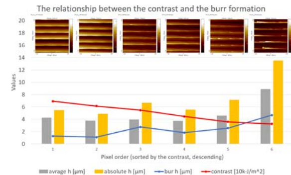
Figure 4. The contrast decreased as the burr heights increased.
