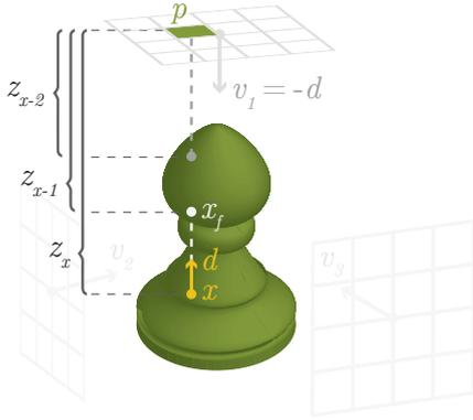
Figure 4: Querying the multi-view LDMs along the ray from  $x$  in direction  $d$ . First, the LDM corresponding to  $d$  is found ( $v_1 = -d$ ). Second,  $x$  is projected into the LDM's view to find  $p$ . Third, the  $(\dots, z_{x-2}, z_{x-1}, z_x, \dots)$  sequence is searched to find  $z_x$ . Fourth, the first intersection along  $d$  is at depth  $z_{x-1}$  from which  $x_f$  can readily be constructed.
