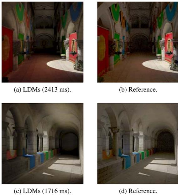
Figure 10: Indirect Lighting. The Crytek Sponza rendered using our approach based on photon differentials traced with LDMs. 512 LDMs of  $200 \times 200$  resolution are used totalling in 805.5 MB of memory. Note that the total render time (in parenthesis) also includes pipeline overhead. Photon tracing takes 2062 ms and 1434 ms in (a) and (c), respectively.
