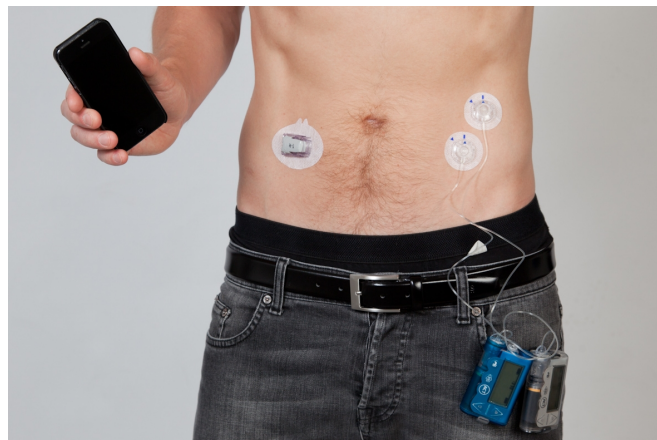
Fig. 1. The dual-hormone artificial pancreas. It includes a CGM sensor, a smartphone for control, an insulin pump and a glucagon pump.
