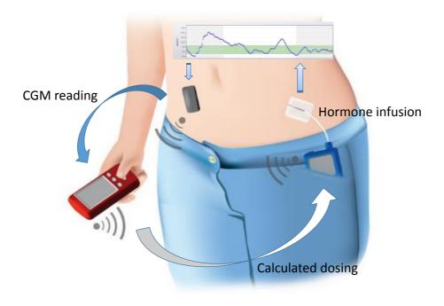
Figure 1.1: Concept of a closed loop artificial pancreas: The CGM measures the glucose concentration, sends it to a control algorithm that determines the hormone dosing, which is then delivered via a pump.
