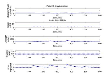
Figure 11: Example of simulated raw data from patient 6 during the medium IIR with first bolus being 75  $\mu$ g. Notice how the glucose infusion is regulated to control the blood glucose close to the set point.
