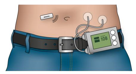
Figure 2.10: The concept of a dual hormone artificial pancreas: infusion sets for insulin and glucagon, sensor for continuous glucose monitoring, and dual chamber pump with insulin and glucagon wirelessly receiving glucose measurements and controlling hormone infusions.
