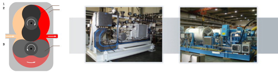
Fig. B.6 Gas Compressors
