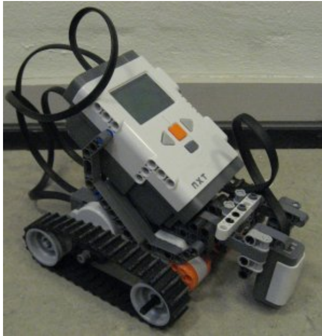
Figure 5.1: The layout of the second iteration robot. The important difference is that the wheels has been switched with caterpillar tracks and that the light sensor have been switched with a color light sensor
