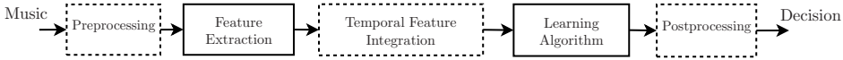
Figure 1.2: The figure shows a flow-chart of a system usually applied for automated music organisation. The solid boxes indicate typical operations performed whereas the dotted boxes are applied by some authors.
