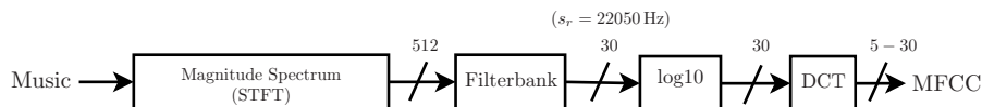
Figure 3.2: The figure illustrates a MFCC extraction scheme. The numbers above each stage expresses the dimension of a typical dimensionality reduction taking place in such a feature extraction stage.
