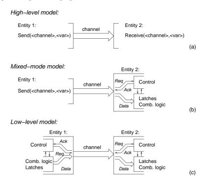
*Figure 8.11.* The VHDL packages for channel communication support high-level, mixed-mode and gate-level/standard cell simulations.
