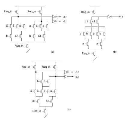
*Figure 5.18.* The CMOS transistor implementation of a full adder for the hybrid adder in figure 5.17: (a) a weakly indicating carry circuit, (b) the sum circuit and (c) a strongly indicating carry circuit.
