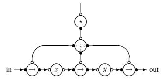
Figure 8.6. The compiled handshake circuit for the 2-place shift register.
