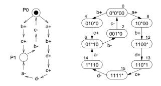
Figure 6.11. The STG specification and the corresponding state graph.
