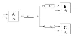
*Figure 2.16.* A circuit fragment with gate and wire delays. The output of gate A forks to inputs of gates B and C.
