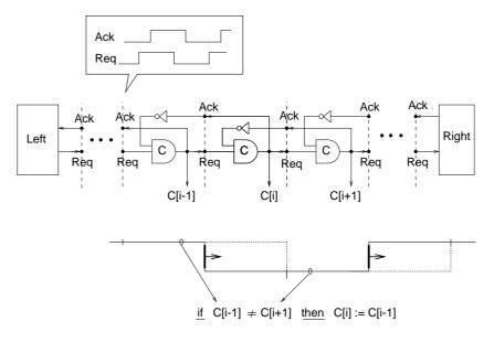
Figure 2.8. The Muller pipeline or Muller distributor.
