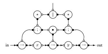
Figure 8.8. Optimized handshake circuit for the FIFO program.
