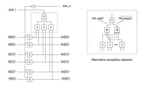
Figure 2.13. An N-bit latch with completion detection.
