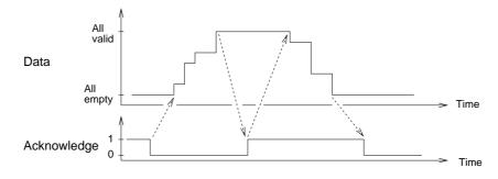
Figure 2.3. Illustration of the handshaking on a 4-phase dual-rail channel.
