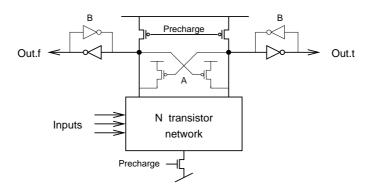
*Figure 5.13.* A precharged differential CMOS combinatorial circuit. By adding the crosscoupled p-type transistors labeled "A" or the (weak) feedback-inverters labeled "B" the circuit becomes (pseudo)static.
