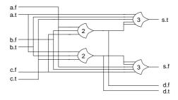
Figure 5.12. A full adder using NCL gates.
