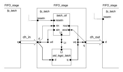
Figure 8.20. Separation of control and data.
