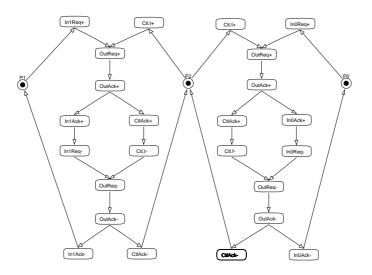
*Figure 6.24.* The STG specification of the control circuit for a 4-phase bundled-data MUX using a 4-phase dual-rail control channel. Combined with the STG fragment for a bundled-data (control) channel the resulting STG for an all 4-phase dual-rail MUX is obtained (figure 6.25).
