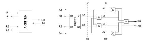
Figure 5.21. The handshake arbiter: symbol and possible implementation.
