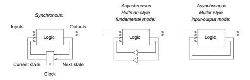
*Figure 6.1.* (a) A synchronous sequential circuit. (b) A Huffman style asynchronous sequential circuit with buffers in the feedback path, and (c) a Muller style asynchronous sequential circuit with wires in the feedback path.
