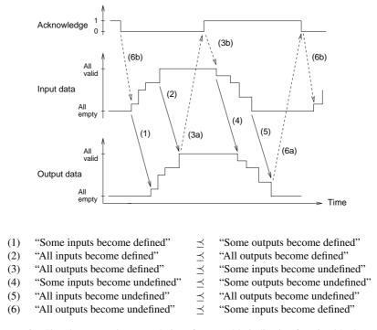
Figure 5.6. Signal traces and event orderings for a weakly indicating function block.
