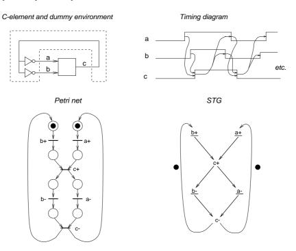
*Figure 6.4.* A C-element and its 'well behaved' dummy environment, its specification in the form of a timing diagram, a Petri net, and an STG formalization of the timing diagram.
