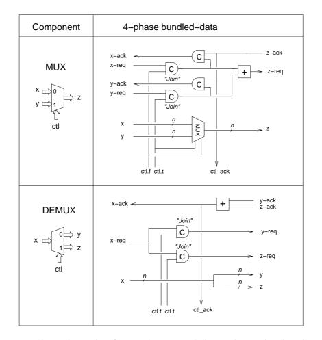
*Figure 5.19.* Implementation of MUX and DEMUX. The input and output data channels x, y, and z use the 4-phase bundled-data protocol and the control channel ctl uses the 4-phase dual-rail protocol (in order to simplify the design).
