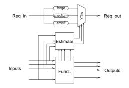
Figure 5.9. The basic idea of "speculative completion".
