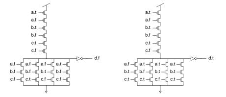
*Figure 5.14.* Transistor-level implementation of the carry signal for the strongly indicating full adder from figure 5.10(c).
