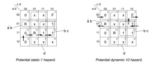
*Figure 6.13.* The Karnaugh maps for output signal c showing state sequences that may lead to hazards.
