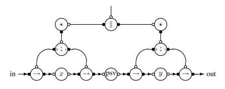
Figure 8.7. Compiled handshake circuit for the FIFO program.
