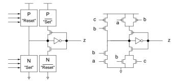
*Figure 6.17.* A generalized C-element: gate-level symbol, and some CMOS transistor implementations.
