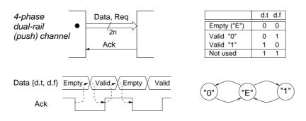
Figure 2.2. A delay-insensitive channel using the 4-phase dual-rail protocol.
