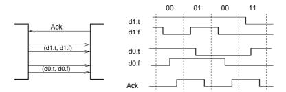
Figure 2.4. Illustration of the handshaking on a 2-phase dual-rail channel.
