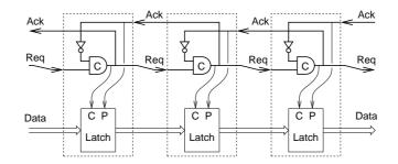
*Figure 2.10.* A simple 2-phase bundled-data pipeline.
