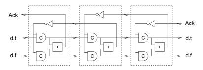
Figure 2.12. A simple 3-stage 1-bit wide 4-phase dual-rail pipeline.
