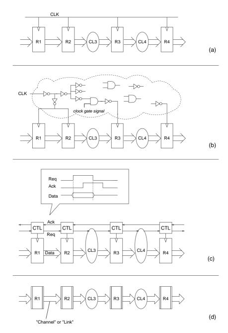
*Figure 1.1.* (a) A synchronous circuit, (b) a synchronous circuit with clock drivers and clock gating, (c) an equivalent asynchronous circuit, and (d) an abstract data-flow view of the asynchronous circuit. (The figure shows a pipeline, but it is intended to represent any circuit topology).
