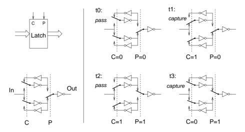
*Figure 2.11.* Implementation and operation of a capture-pass event controlled latch. At time  $t_0$  the latch is transparent (i.e. in pass mode) and signals C and P are both low. An event on the C input turns the latch into capture mode, etc.
