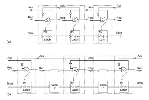
Figure 2.9. A simple 4-phase bundled-data pipeline.
