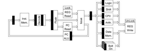
Figure 3.13. Architecture of the ARISC microprocessor.
