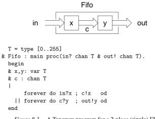
Figure 8.3. A Tangram program for a 2-place (ripple) FIFO.
