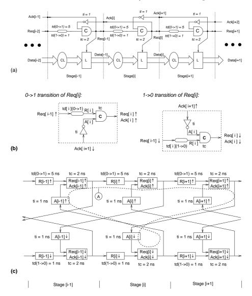
*Figure 4.7.* Data dependency graph for a 3-stage section of a pipeline: (a) the circuit diagram, (b) the two graph fragments corresponding to a pipeline stage, and (c) the resulting data-dependency graph.
