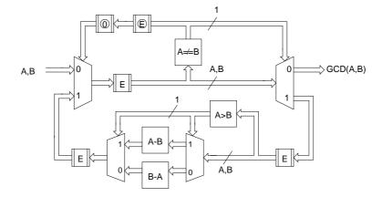
Figure 3.12. An asynchronous circuit implementation of GCD.
