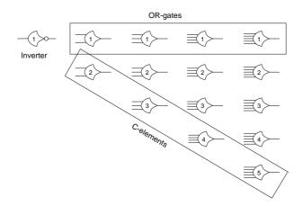
*Figure 5.11.* NCL gates: m-of-n threshold gates with hysteresis ( $1 \le m \le n$ ).
