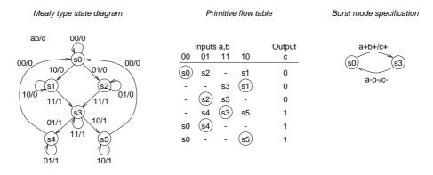
*Figure 6.3.* Some alternative specifications of a Muller C-element: a Mealy state diagram, a primitive flow table, and a burst-mode state diagram.
