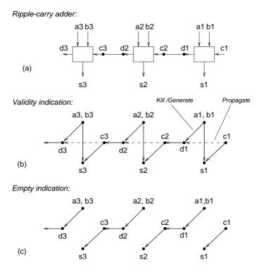
*Figure 5.15.* (a) A 3-stage ripple-carry adder and graphs illustrating how valid data (b) and empty data (c) propagate through the circuit (Martin [61]).
