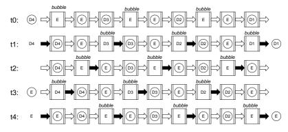
*Figure 4.1.* A FIFO and its environment. The environment alternates between reading a token from the FIFO and writing at token into the FIFO.
