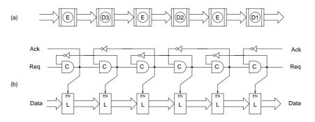
*Figure 7.4.* (a) A FIFO based on handshake latches, and (b) its implementation using simple latch controllers and level-sensitive latches. The FIFO fills with valid data in every other latch. A latch is transparent when EN = 0 and it is opaque (holding data) when EN = 1.
