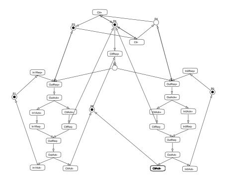
*Figure 6.25.* The final STG specification of the control circuit for the 4-phase bundled-data MUX. All channels, including the control channel, are 4-phase bundled-data.
