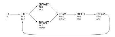
*Figure 8.13.* The protocol for the abstract channel. The values in large letters are the resulting resolved values of the channel, and the values in smaller letters below them are the driving values of the sender and receiver respectively.
