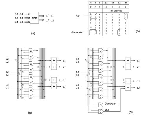
*Figure 5.10.* A 4-phase dual-rail full-adder: (a) Symbol, (b) truth table, (c) DIMS implementation and (d) an optimization that makes the full adder weakly indicating.
