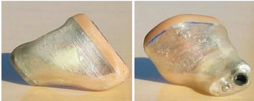
Figure 8.3: SLA print of the minimum shell with the faceplate, tipplate, and components added.
