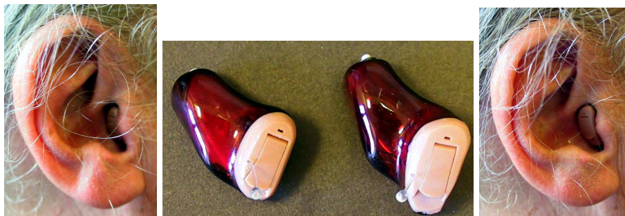
Figure D.2: Two CIC hearing aids made for the same ear canal. It is seen that the left CIC is smaller than the one to the right. The size difference is mainly due to the placement of the faceplate. It is seen that the visual appearance of the hearing aid in the ear is strongly influenced by the size.
