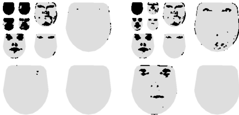
Figure 8.6: Selected wavelet coefficients for the face training set (CDF, ratio 1:10). The scaling coefficients are shown in the upper left. Left: \|\mathcal{W}\|_2 = 1 . Right: \|\mathcal{W}\|_2 = 1/\sqrt{2} .
