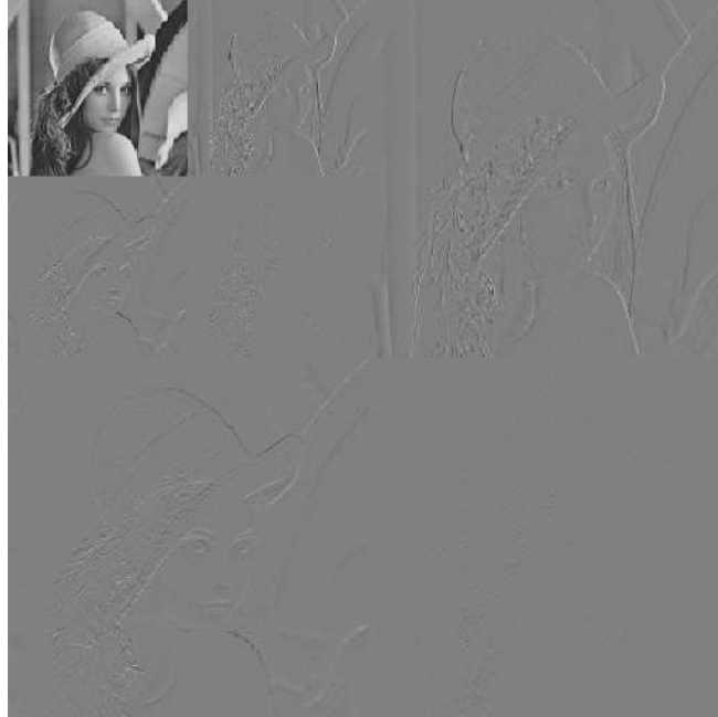
Figure 8.1: The wavelet coefficients of a two-level octave decomposition using the Haar wavelet.
