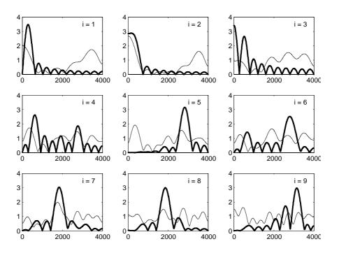
Figure 5: Frequency responses  $|\hat{v}_i(f)|$  and  $|\hat{v}_i(f)|$  of the FIR filters for the SVD algorithm (thick lines) and the hulv-version of the ULV algorithm (thin lines).
