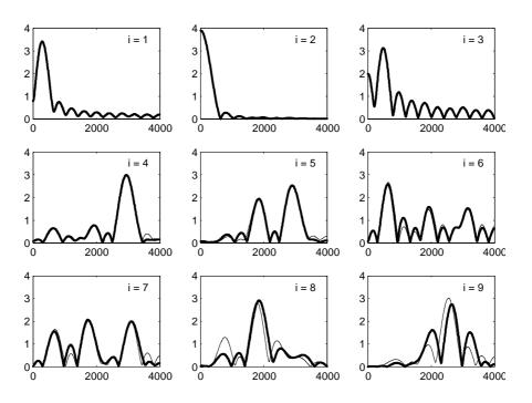
Figure 4: Frequency responses  $|\widehat{w}_i(f)|$  and  $|\widehat{\overline{w}}_i(f)|$  of the canonical FIR filters for the truncated SVD and ULV algorithms. Thick lines: SVD filters; thin lines: ULV filters.
