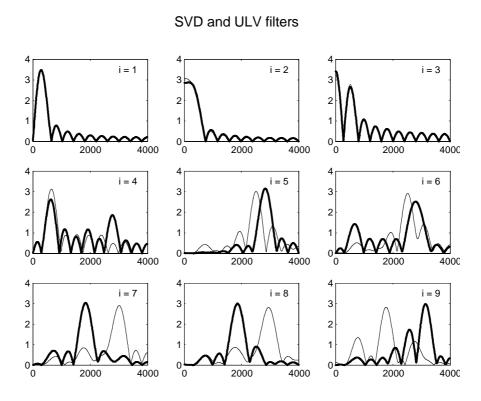
Figure 2: Frequency responses  $|\widehat{v}_i(f)|$  and  $|\widehat{v}_i(f)|$  of the FIR filters for the truncated SVD algorithm (thick lines) and the truncated ULV algorithm (thin lines), defined via the vectors  $v_i$  and  $\overline{v}_i$  for  $i=1,\ldots,9$ .
