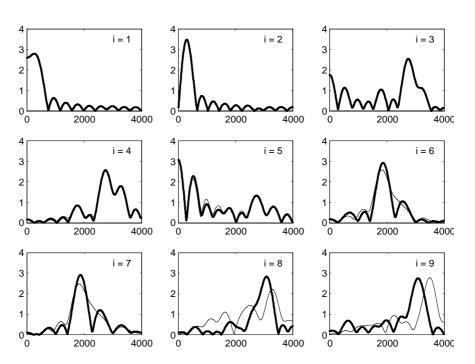
Figure 6: Frequency responses  $|\widehat{w}_i(f)|$  and  $|\widehat{\overline{w}}_i(f)|$  of the canonical filters for the SVD algorithm (thick lines) and the hulv-version of the ULV algorithm (thin lines).
