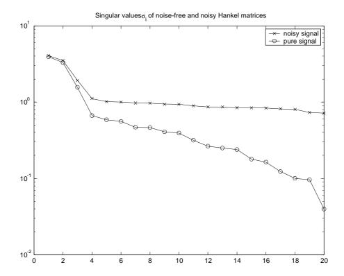
Figure 1: Singular values  $\sigma_i$  of the Hankel matrix  $A = \mathcal{H}(x)$  corresponding to a pure and a noisy signal vector x.
