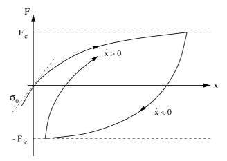
Fig. 3: Sketch of the friction force F as a function of the dissaplacement x.
