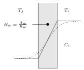
Fig. 8: Model approximations for the conductive heat transfer through a wall.
