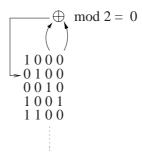
Figure 2.3: Generation of a PRBS sequence, exemplified using a shift register circuit with n=4. In the first step a zero is generated (0+0 mod 2=0). The generated number is put back in the shift register. In the second step, a new zero is generated (0+0 mod 2=0) followed by a one in the next step (1+0 mod 2=1) etc.
