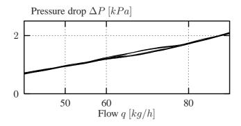
Fig. 6: Phase diagram of the pressure drop  $\Delta P$  vs. the flow q.
