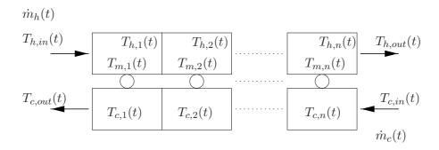
Fig. 5: The compartmental counter flow heat exchanger model.
