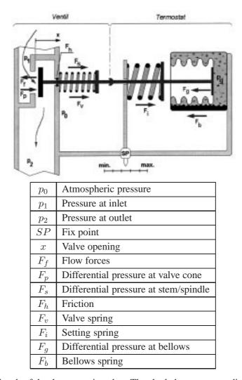
Fig. 1: Sketch of the thermostatic valve. The shaded area surrounding  $p_q$  indicates the gas chamber, while the arrows at  $p_1$  and  $p_2$  indicates the upstream and downstream pressure. The nomenclature for the various parameters are given in the table below the sketch.
