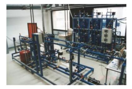
Figure 2.4: Experimental setup at the Danish Technological Institute. The heating system corresponds in capacity to 20 apartments, consisting of three water tanks, heat exchangers, valves, pumps and pipes as well as data acquisition equipment.
