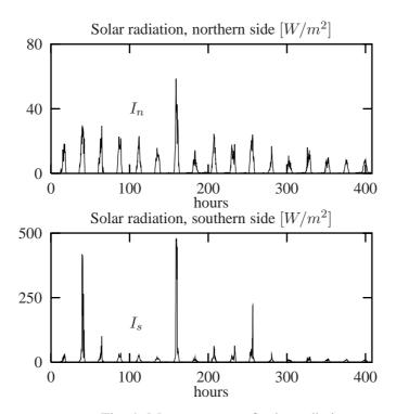
Fig. 4: Measurements of solar radiation.
