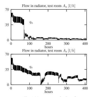
Fig. 5: Measurements of radiator flow.
