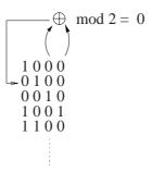
Fig. 2: Generation of a PRBS sequence, exemplified using a shift register circuit with n=4. In the first step a zero is generated (0+0 mod 2=0). The generated number is put back in the shift register. In the second step a new zero is generated (0+0 mod 2=0) followed by a one in the next step (1+0 mod 2=1) etc.
