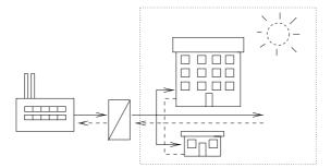
Fig. 1: Sketch of a typical DH system. The combined heat and power plant supplies the consumer via heat exchangers with hot water (solid line) for heating and domestic water. After consumption, the cooled water (dotted line) returns to the power plant.
