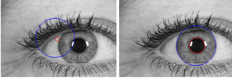
Figure 3.6: Left: Result obtained without a mask to account for the reflections. Right: Result obtained with a mask accounting for the reflections
