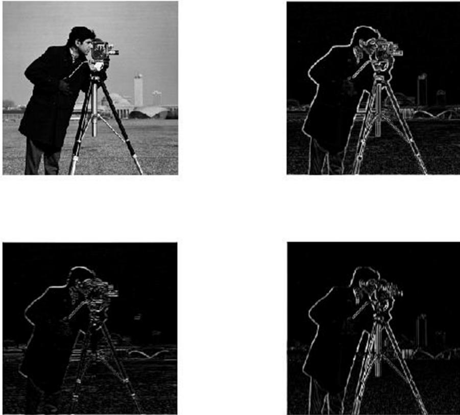
Figure 3.11: Upper left: original image, upper right: Gradient magnitude, lower left: Vertical derivative using Prewitt filter, lower right: Horizontal derivative using Prewitt filter
