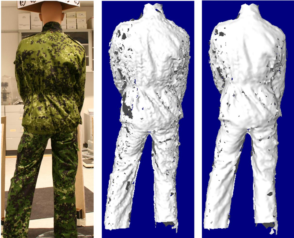
Figure 1.27: Left: Photo; Center: Triangulated mesh without processing<sup>3</sup>; Right: Processed triangulated mesh
