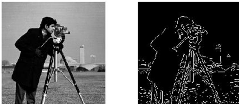
Figure 3.14: Results of an edge detection using a LoG filter. Left: original photo; Right Photo Labeling of zero crossings in the LoG filtered photo.
