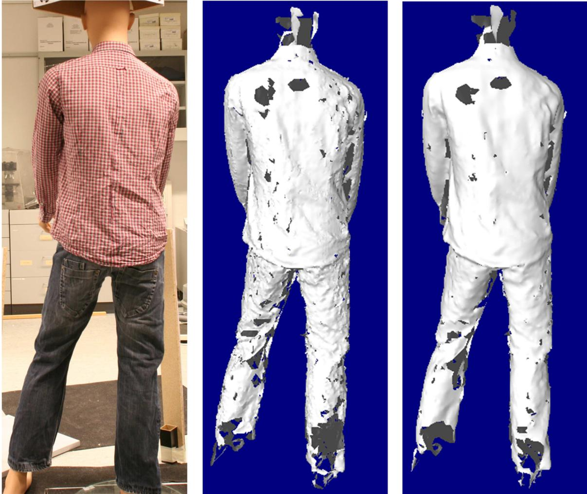
Figure 1.28: Left: Photo; Center: Triangulated mesh without processing<sup>4</sup>; Right: Processed triangulated mesh
