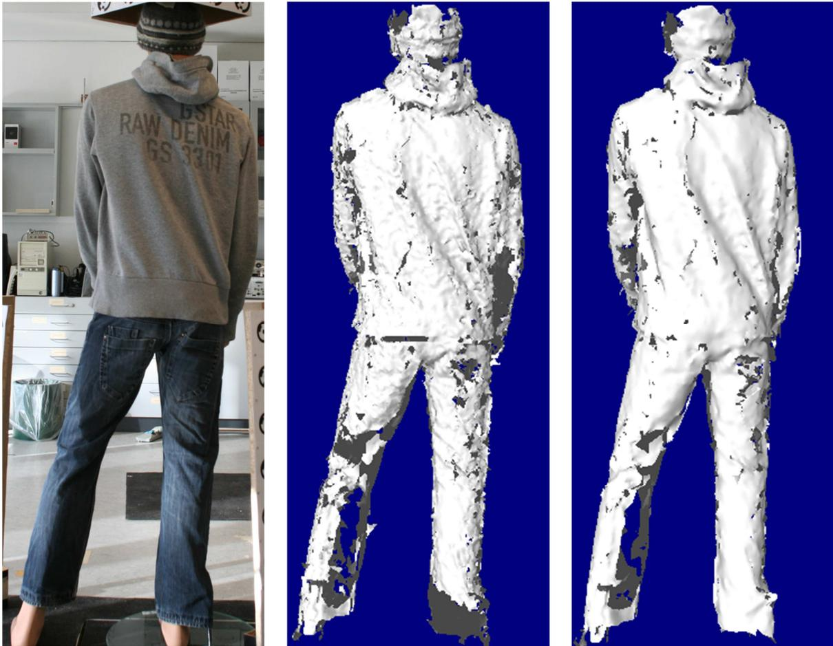
Figure 1.29: Left: Photo; Center: Triangulated mesh without processing<sup>5</sup>; Right: Processed triangulated mesh
