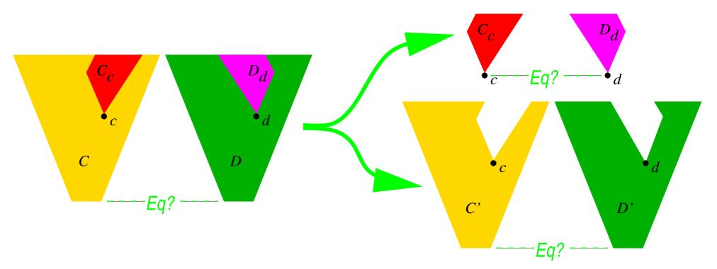
Given *conjectured* equivalence between nodes c and d of circuits C and D,
