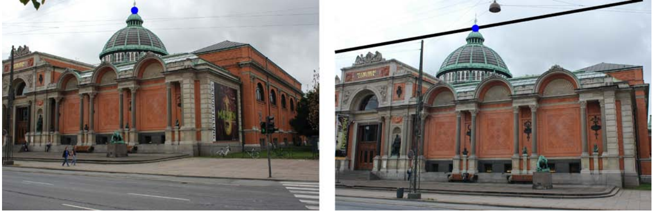
Figure 2.4: An image pair, with image one to the left and image two to the right. A point, \mathbf{q}_1 , is annotated in image one (blue dot). The corresponding epipolar line, l_2 , and 2D point, \mathbf{p}_2 is annotated in image two. This is done by the black line and blue dot respectively.
