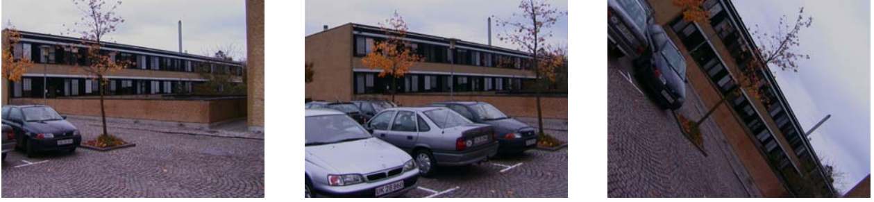
Figure 4.4: Three images of a building here at DTU. It is relatively easy to match the left and middle image via correlation, since the image motion is moderate and there is no or little rotation. Matching the left and right image will likely give problems using correlation due to the large amount of rotation.
