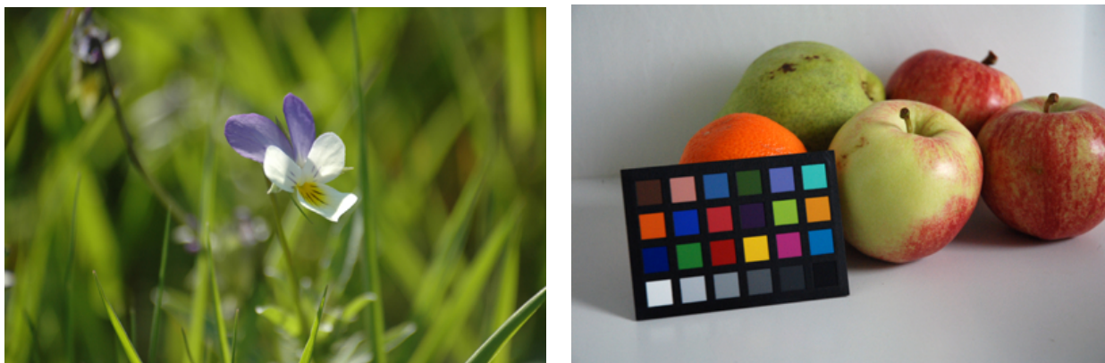
Figure 1.23: Left: Example of depth of field of a camera, note that it is only the flower and a couple of straws that are in focus. Right: Example of a color calibration card. These colors of the squares in the card are very well known. As such the image can be chromatically calibrated.
