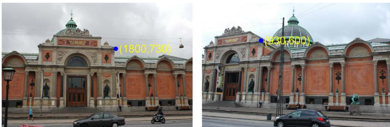
Figure 2.12: Two images with known camera models. Two points corresponding to the same 3D point have been annotated, such that this 3D point can be estimated.
