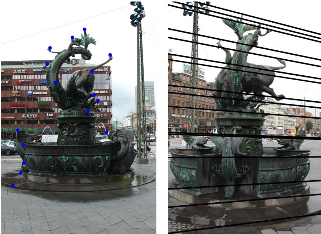
Figure 2.6: A collection of epipolar lines in the right image one for each point in the left image. It is seen that all the epipolar lines form a bundle intersecting in the same point, i.e. the epipole.
