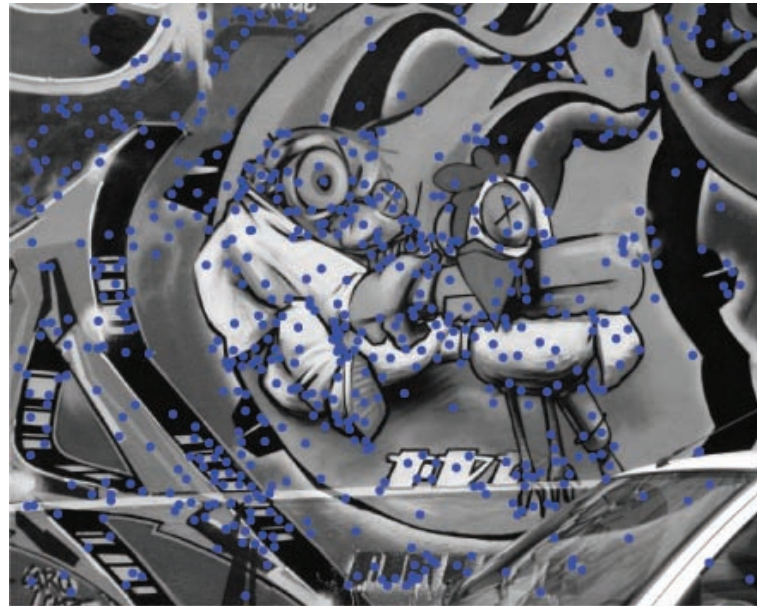
Figure 3.14: An example of extracting the DoG features across scale corresponding to the so-called SIFT features [20].
