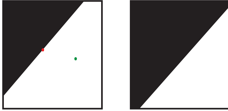
Figure 3.6: An illustration of the aperture problem. Two features (the red and green dots) are annotated in the left image. Consider finding these features in the right image, given that this image is a slightly transformed version of the left. The red dot – located on the line – must be located on the line in the right image, although it is undetermined where. As for the location of the green dot, all we can say is that it must be located in the white area of the right image. This illustrates that we can only uniquely determine the position of a feature in the direction of image gradients.
