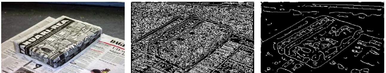
Figure 3.2: The maximum of the gradient magnitude is computed for the leftmost image and depicted in the middle and right images. The difference between the middle and right image is the scale at which the gradient is computed. Notice how different structures appear at the different scales.
