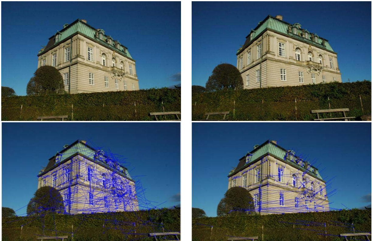
Figure 4.6: An example of the correspondence problem, where the two top images are to be matched. Features are extracted as Harris corners, and matched via correlation. In the bottom row the blue arrows indicates the displacements needed to get a match. On the left is an unconstrained matching, whereas the camera geometry is used to the right.
