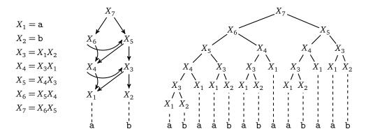
Figure 1: An SLP compressing the string abaababaabaab, its corresponding DAG, and its parse tree.
