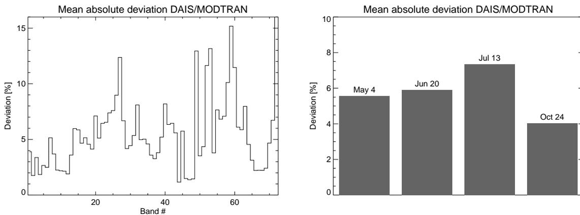
Figure 6. Mean deviations of DAIS measurements from MODTRAN predicted radiances
