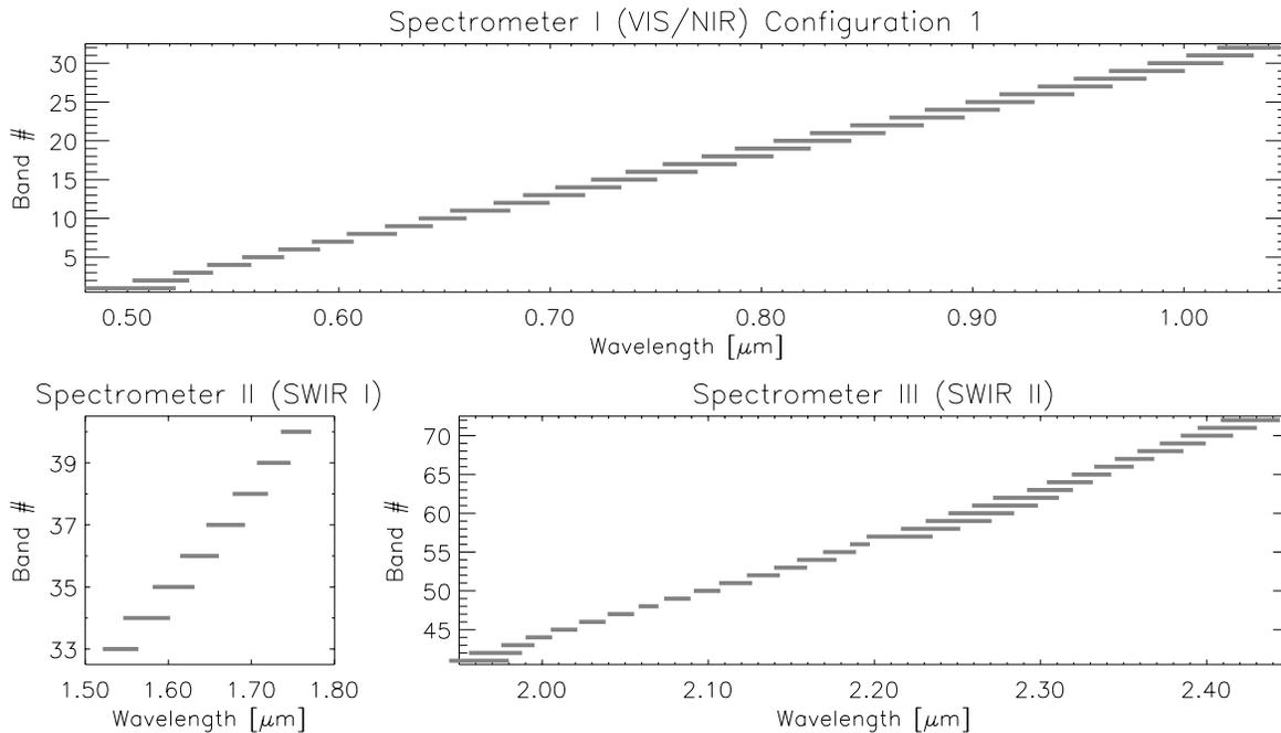
Figure 1. Bandposition and bandwidth in the first three spectrometers of the DAIS 7915
