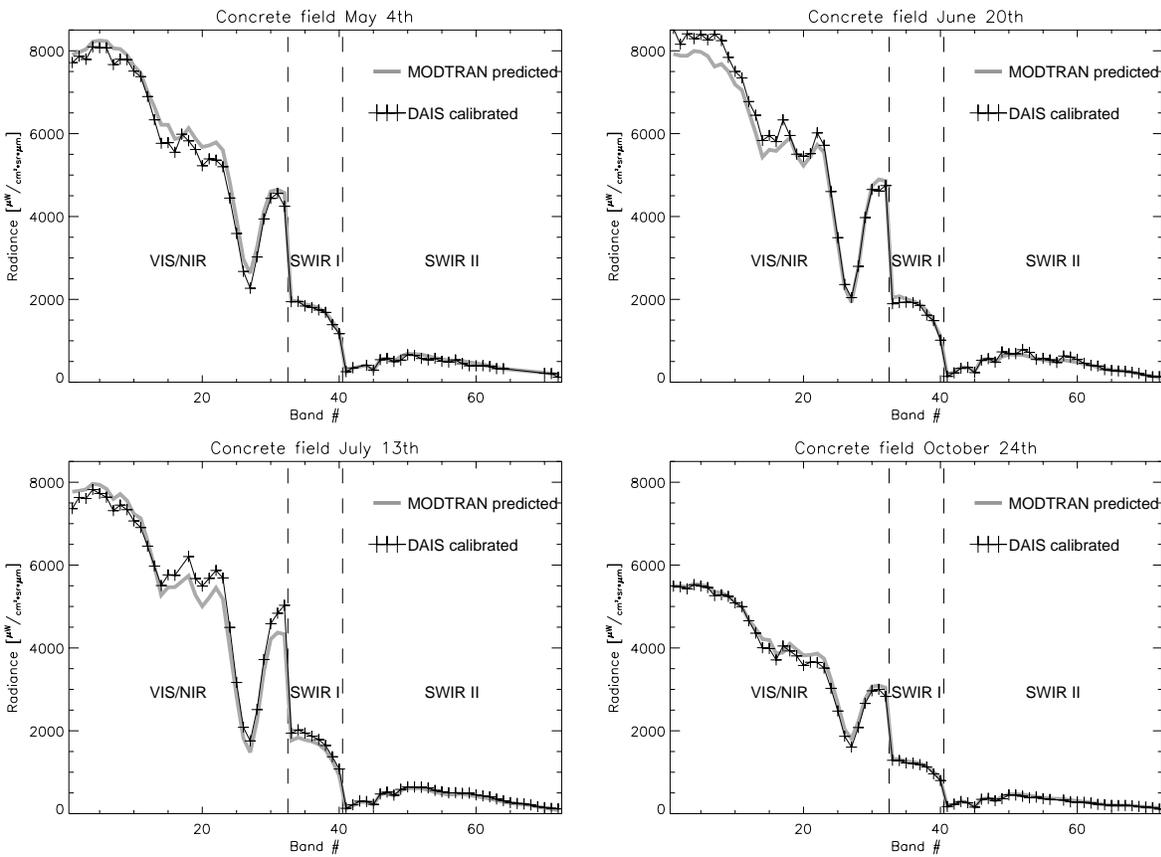
Figure 5. DAIS measured and MODTRAN predicted at sensor radiance for the inflight validation dates.
