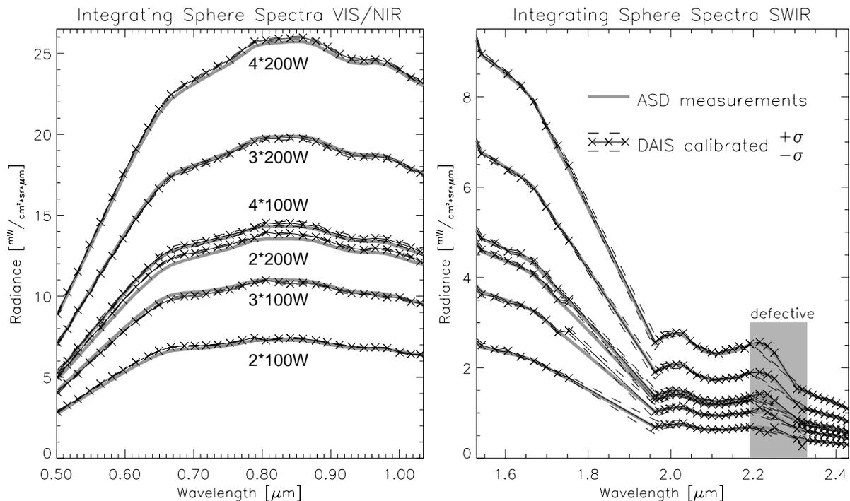
Figure 2. Measured radiance spectra and DAIS calibrated data acquired on the integrating sphere were resampled to the DAIS bands using a convolution algorithm and the DAIS response curves obtained by the spectral calibration part (SCP) (Oertel, 1994). These resampled radiance spectra serve as the reference for the DAIS calibration, they are given in Figure 2.
