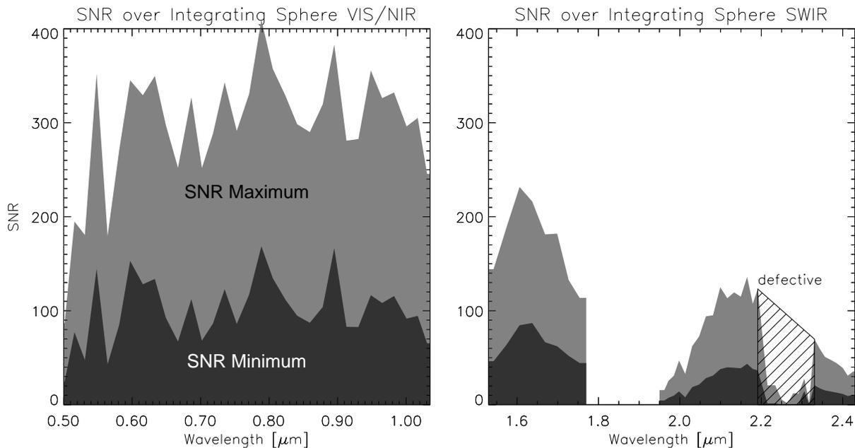
Figure 3. Signal to Noise Ratios calculated from entire scenes acquired on the integrating sphere
